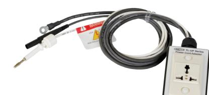
The TL-UP2 Test Adaptor allows for easy Hipot and Ground Bound connection to virtually any device with a power cord. The TL-UP2 routes high voltage to both the line and neutral pins of the power socket and connects the earth pin of the socket to the return of the tester. A separate test lead can be connected to the DUT chassis for continuity or Ground Bond testing to the earth pin of the DUT power cord. Available in Hipot/Continuity or Hipot/ Ground Bond versions.
